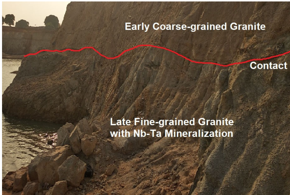
Figure 6-3 Wall of Open Pit Showing the Contact between Early Coarse-grained granite and Late Fine-grained Granite
